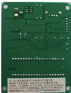
STC12/11/10/89/90系列40-pin单片机ISP下载编程工具反面
